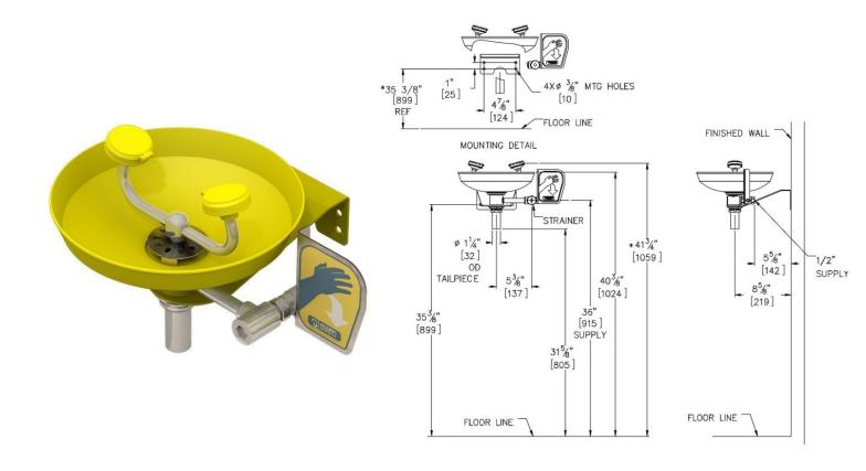
Model S0420 is a wall mounted eye/face wash, with a plastic bowl, ABS plastic eye/face wash spray heads, an inline strainer and a stay-open 1/2" ball valve with a push handle. Comes complete with safety sign and weekly testing card as per ANSI Z358.1 compliance.
